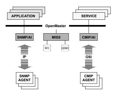
OpenMaster enforces a CMIP vision of the network. The agent integrators translate the operations on the network elements and convert the event notifications in a normalized form.
